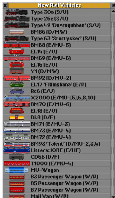
**Description:** it consists of vehicle code (e.g. BM93), name (e.g. 'Talent'), traction type (S=steam, D=diesel, E=electric) and usage class (U=universal, P=passenger, F=freight, HF=heavy freight, MW=motorised wagon, MU=multiple unit). The number at the end of a Multiple Unit (MU-n) description indicates how many vehicles including engine(s) should or could make up a train.
